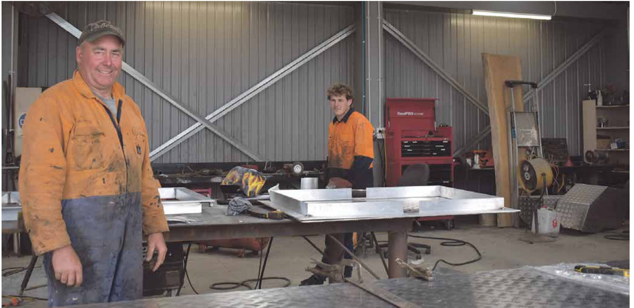
Ben Carson, left, and Hunter Knott working on aluminium drain covers at Carson Engineering.
