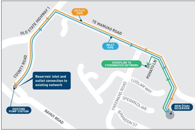
A map showing the location of pipes to and from the reservoir.
