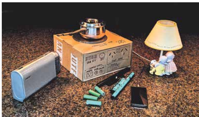
BOX ON THE GO: A prototype of Dave Timperley's Go Box, a portable electricity storage unit built from recycled laptop batteries. Photo supplied
