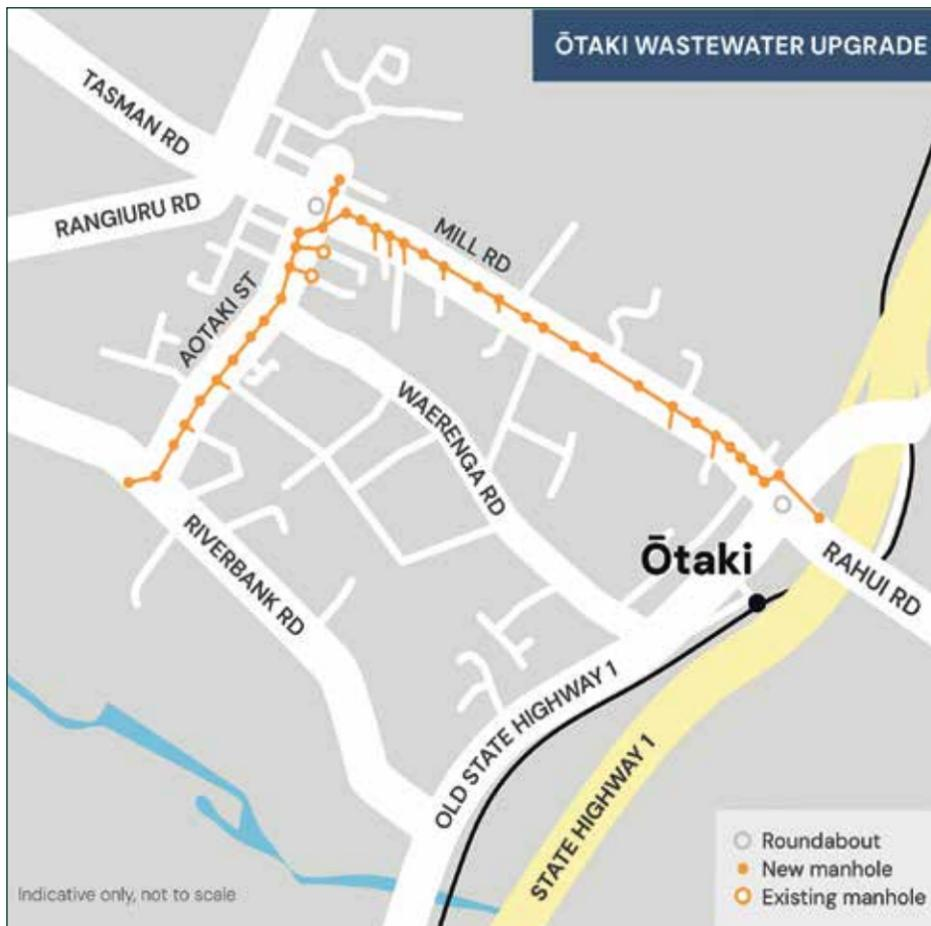
A KCDC map showing where 2.7km of pipes will be laid to increase the capacity of the town's wastewater system.
