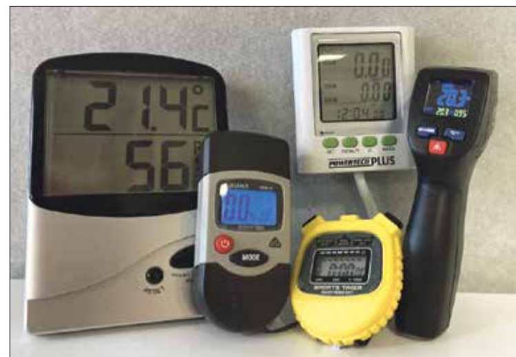
KITS: The Healthy Home Kits available at Ōtaki Library contain a thermometer/hygrometer, a wood moisture meter, a power meter, a stopwatch, and an infrared thermometer. Photo supplied
